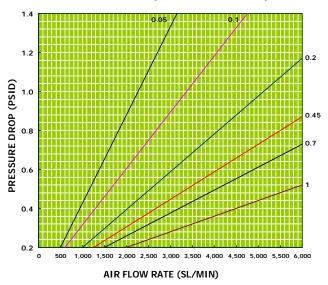
Air Temperature: 24 °C, Inlet Pressure: 15 PSID (1 Bar)
